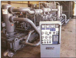
■ A view of the fully pneumatic control panel as delivered from customer (left). The remanufactured Superior 16SGT-MW66 package (right) was customized with a fully electronic Altronic EPC 200c digital control system and a one-year "new unit" warranty.
